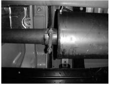
REMOVE THE FIRST CLAMP IN FRONT OF YOUR MUFFLER AND REMOVE STOCK EXHAUST. DO NOT REMOVE EXTENSION PIPE BETWEEN MUFFLER AND CATALYTIC CONVERTER.
