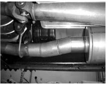
INSTALL HEADPIPE #A USING CLAMP #G TO ATTACH IT TO THE STOCK HEADPIPE
