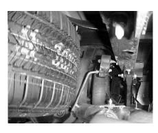
INSTALL DRIVERSIDE TAILPIPE #C TO OUTLET OF MUFFLER AND INSERT WELDED HANGER INTO RUBBER GROMMET. ATTACH TO MUFFLER WITH CLAMP #F. DRIVERSIDE TAILPIPE #C BRACKET SHOULD BE ON TOP OF TAILPIPE #D BRACKET. BOLT TAILPIPES TOGETHER USING BOLT KIT #I. DO NOT TIGHTEN UNTIL SYSTEM IS POSITIONED WITH 1" CLEARANCE FROM FRAME AND SHOCKS.
